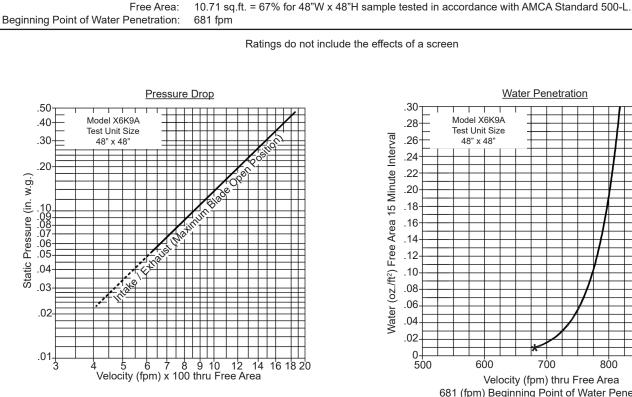
The AMCA Certified Ratings Seal applies to Air Performance only. Tested in accordance with AMCA Standard 500-L, Test Figure 5.5 - 6.5
